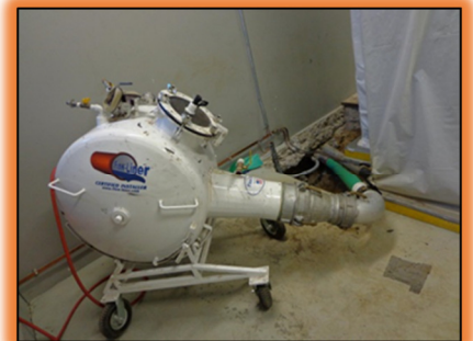
Flow-Liner® Equipment Set-up
